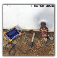
PEC TANK FLOOR Allows for the inspection of a tanks critical zone corrosion externally. No need to empty or shut down a tank for entry.
