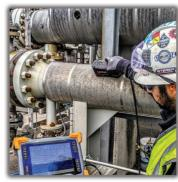
**PEC SINGLE-ELEMENT** For optimal penetrating power, the single-element probes can be utilized on any application providing the highest data resolution possible.
