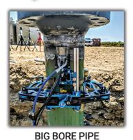
Great for piping 6" and greater; i.e. pipeline and power projects, as well as fab. and field welds. Equipment capabilities include TOFD, TFM, and FMC.
