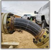
**BIG-BORE PIPE + ELBOWS** By utilizing ultrasonics, ICM works on any material type and schedule. From small-bore pipes to big-bore elbows, any asset can be inspected.
