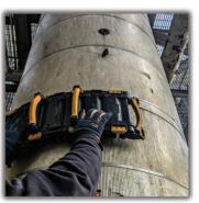
**PEC-ARRAY** With 6x built-in channels, this probe is perfect for piping 6" or greater, vertical or horizontal vessels, and tank shells.
