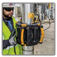
**PIPE + VESSELS + TANKS** Works on a variety of material and insulation combinations. Custom probes are available for more specialized projects.
