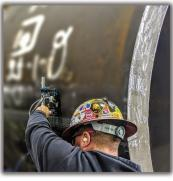
THICK MATERIAL Ideal for thicker materials due to the penetrating power of PAUT. Eliminates the need for dangerous cobalt sources.
