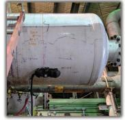
SEPARATORS + VESSELS When entry for inspection is not permitted, scanning from the OD with the compact probe can provide up to 100% coverage of an area's ID & OD.
