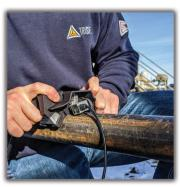
SMALL-BORE PIPE Specialized PAUT probes and encoders allow for piping scans down to 2" in diameter, regardless of material type or schedule.
